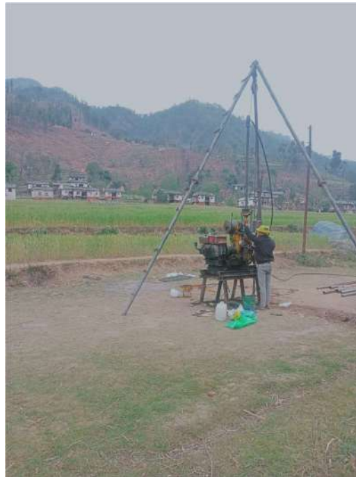
Figure 5 Instrument setup for Standard Penetration Test
