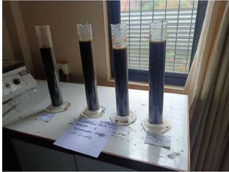
Figure 7 Hydrometer analysis conducted at the GTAA Laboratory.
