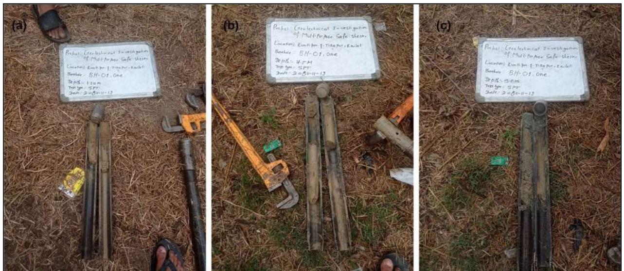
Figure 21 SPT Samples in Borehole-01 in Kailali Site (a) 1.50m (b) 4.50m (c) 9.0m
