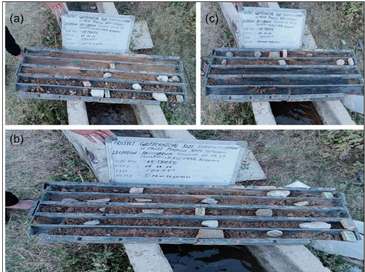
Figure 20 Samples in Borehole-03 in Achham Site (a) 0-5m (b) 5-10m (c) 10-12m
