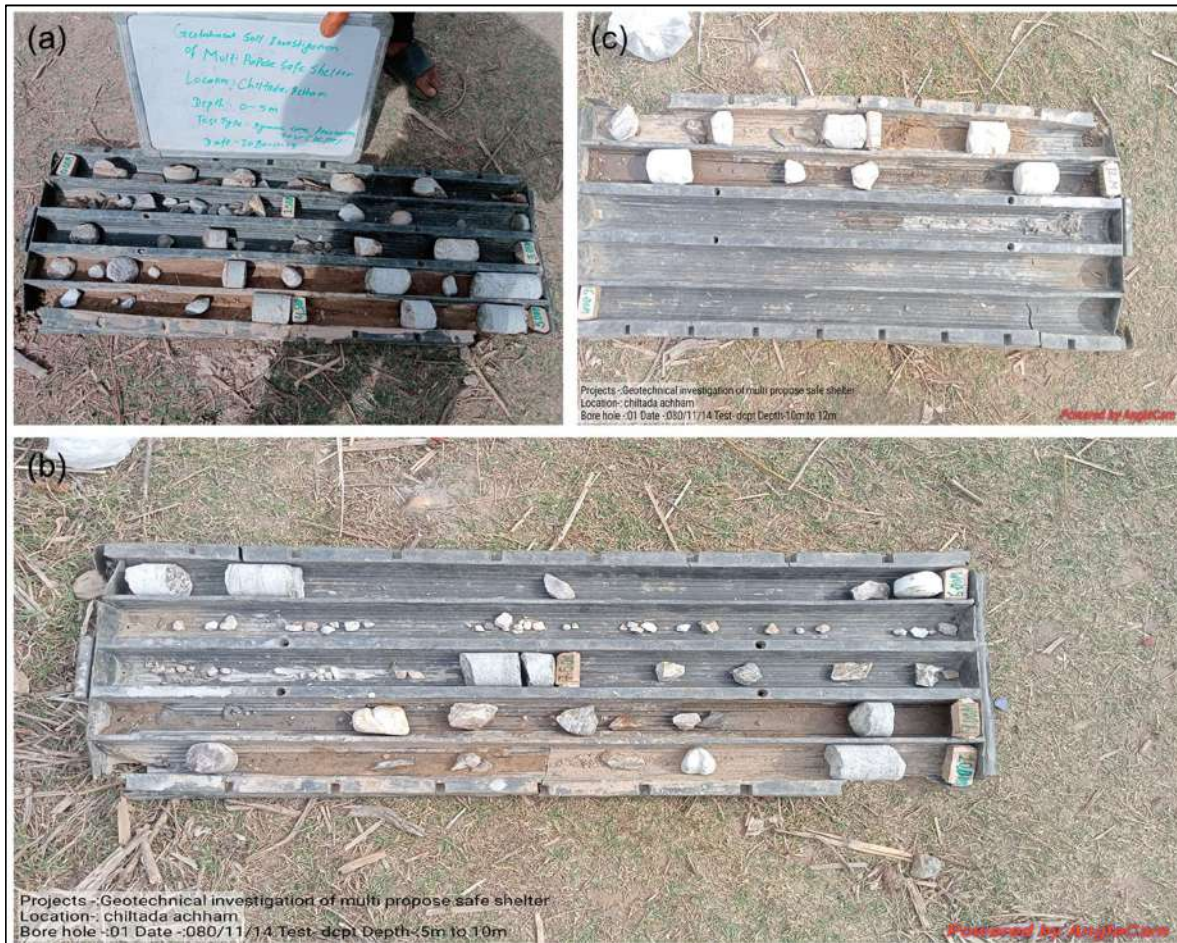
Figure 18 Samples in Borehole-01 in Achham Site (a) 0-5m (b) 5-10m (c) 10-12m
