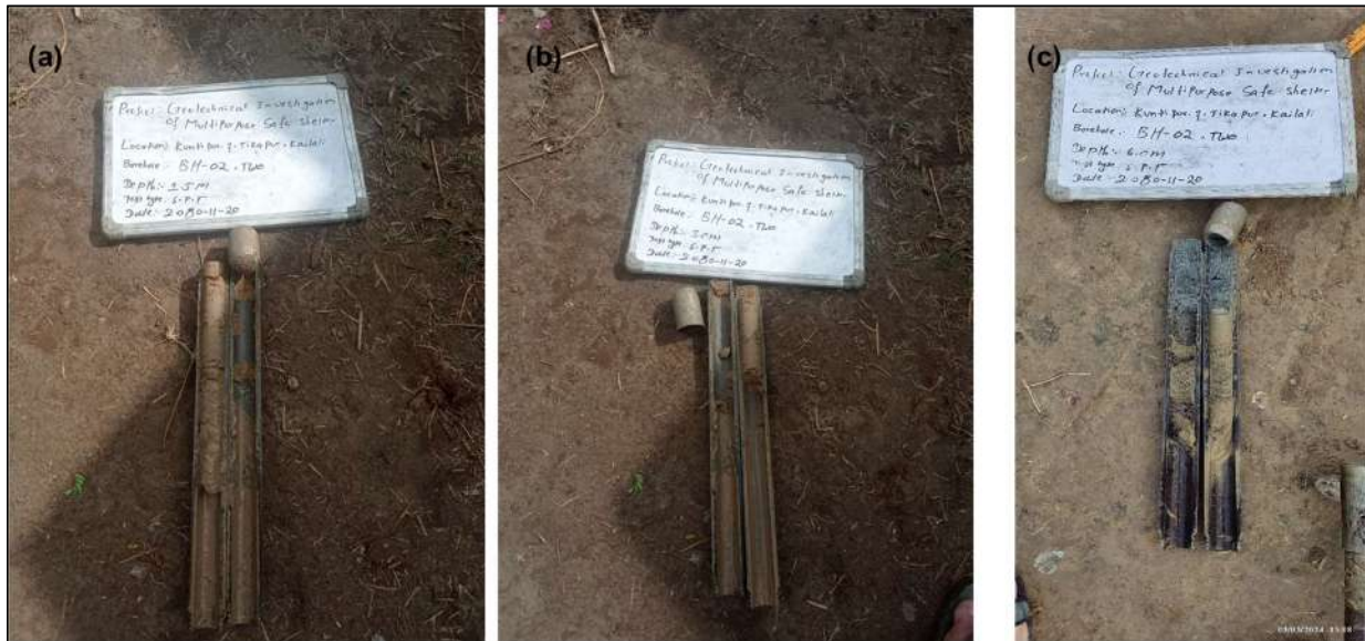
Figure 22 SPT Samples in Borehole-02 in Kailali Site (a) 1.50m (b) 3.0m (c) 6.0m
