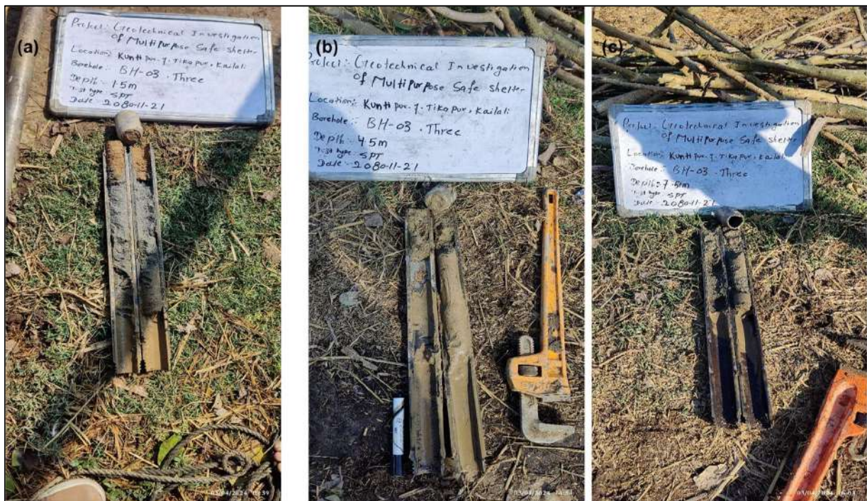
Figure 23 SPT Samples in Borehole-03 in Kailali Site (a) 1.50m (b) 4.50m (c) 7.5m
